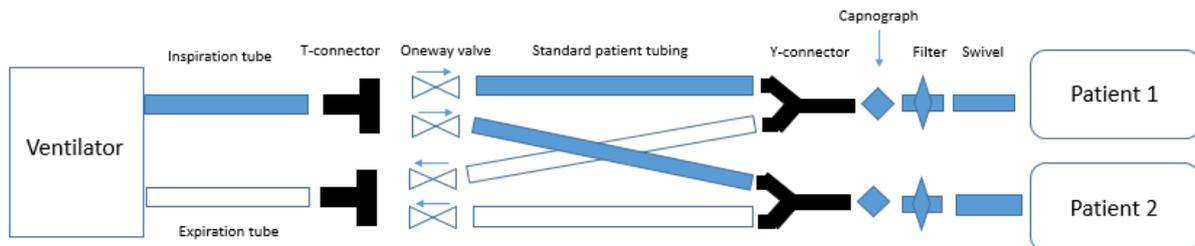
There are 4 one-way-valves required for a circuit with two patients. It is extremely important to verify that the one-way-valves are positioned in the right direction. The circuit should be tested with test lungs before connecting patients.
