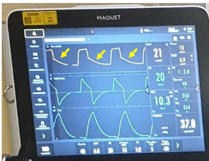
Figure 8 Unusual expiratory flow waveforms caused by using one-way-valves (arrows). Expiratory pressure requires more time than usual to return to the PEEP level because of the increased expiratory resistance in the circuit.
