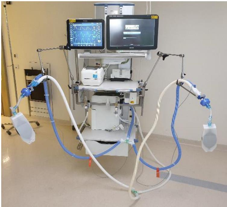
Figure 7 Set-up in practice. Every test lung represents 1 patient. The tidal volumes visible on the ventilator are the total tidal volume of the two test lungs in total.
