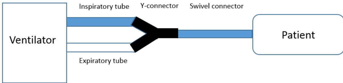
Figure 1 Standard set-up for invasive mechanical ventilation
