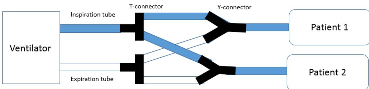
Figure 2 Schematic view how to attach 2 patients to 1 ventilator. One-way-valves are not shown in this figure
