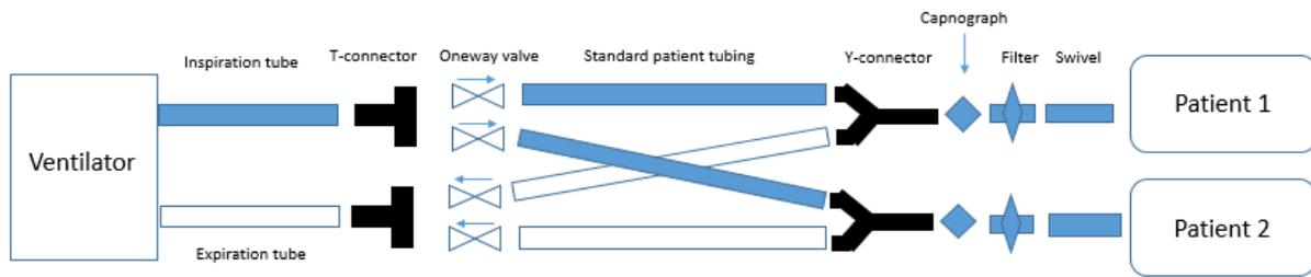
Figure 6 Schematic set-up. The arrows on the T-connectors indicate the direction in which airflow is unobstructed; airflow in the other direction is blocked. See supplement 1 for this figure in more detail and for an option without T-connectors with built-in one-way-valve.
